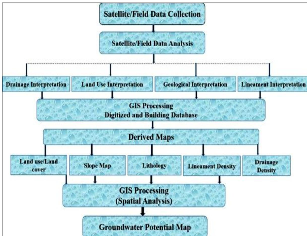
Figure 2: Methodology flowchart for the groundwater potential zone
