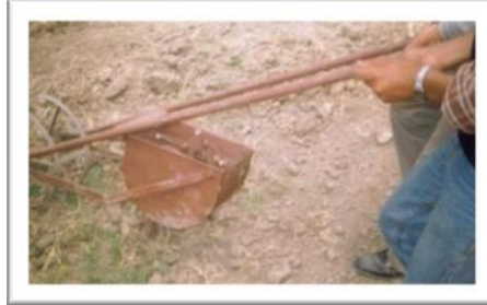
Fig 2. Working of maize planter
