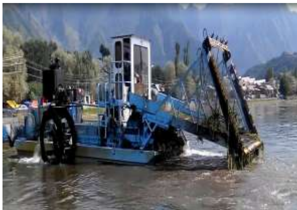
Figure 1: Mechanical harvesters (Aquarius systems) in Dal Lake.
