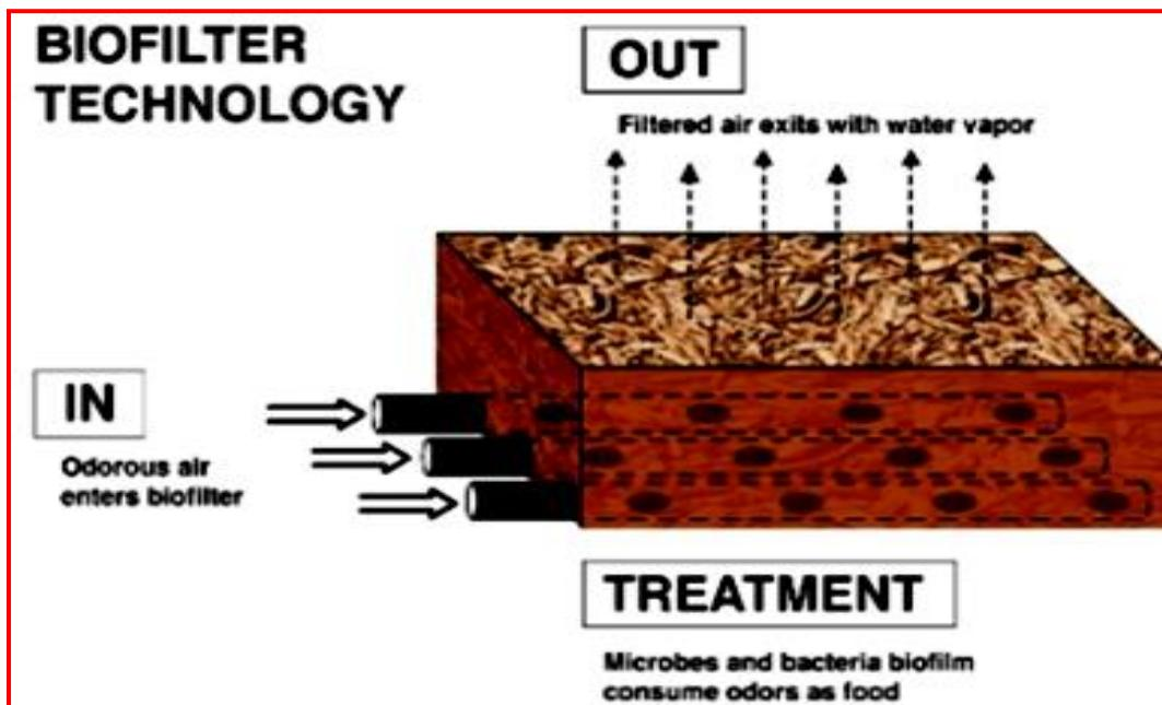
Figure 6: Biofilter technology using biofilms (<http://www.seminarstoptics.com/seminar/8015/biofilters-for-air-pollution-control/>)
